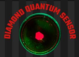
We acquired a nitrogen-rich, lab-grown diamond and made quantum color centers by irradiating the diamond with high-energy neutrons in UW's nuclear reactor. This process was followed by annealing the diamond at high temperature. This approach significantly increased the number of color centers, which improves the signal strength and sensitivity of the magnetic field sensor.
